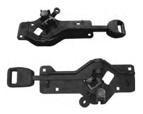
The Design 10 Switch Stand is intended for rails weighing up to 60 lbs per yard. It weighs 38 lbs and can be paired with either a Design 8 spring connecting rod or a Design 8 rigid connecting rod. The Design 11 Switch Stand is for rails weighing 60 lbs per yard or more. It includes locking ears so the lever can be padlocked in either position. Weighing 70 lbs, it can be used with a Design 9 spring connecting rod or a Design 10 rigid connecting rod.
