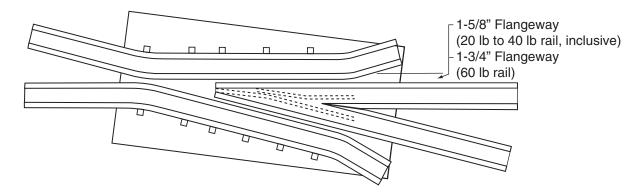
The Welded Plate Frog, Design 97, is recommended for applications in mining, construction, and industrial facilities where lighter rail sections are in use.
