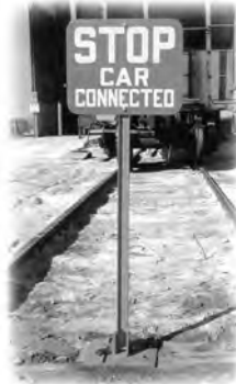
Spike-Down Hinged Tie plate base is spiked to tie. Hinged sign holder folds down. Weight 16 lbs
