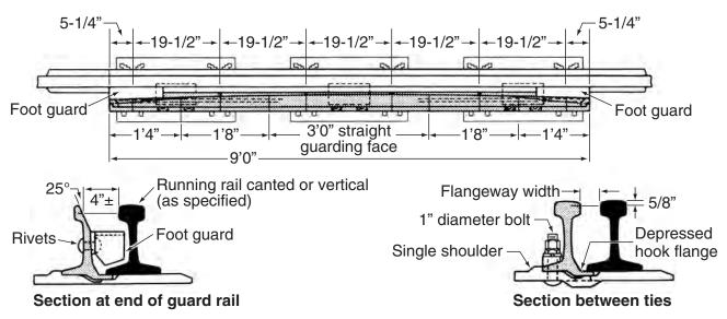
**Manganese one-piece guard rails** (below) consist of a single casting of manganese steel with a reinforced head and corrugated web. They come in a variety of lengths and are marked with the year cast and the height of the guard rail.
