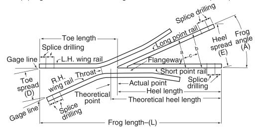
To ensure proper track performance, the frog angle must be appropriate for the curve radius. Several rules and straightforward formulas, which do not require trigonometry, can be used to avoid guesswork when choosing the right frogs for different curves. The formulas below offer good approximations.
