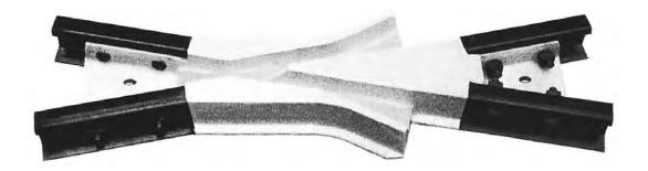
Design 289 is of one-piece construction, made of cast manganese steel. Being of one piece, it has no rivets or plates to work loose. It may be quickly installed, and will outwear several plate frogs. No splice bars are required, the rails being bolted directly to the plate arms, and special long heat-treated bolts with beveled washers are furnished where necessary. Frogs are made with 1/2 inch points.
